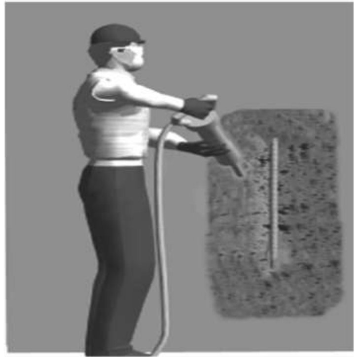
Marking perimeter of the repair area followed by cleaning of the rusted reinforcement bars
